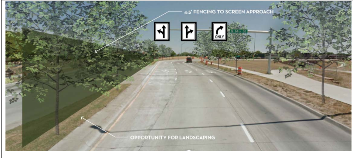
Figure 5: Concept approach screening placed within splitter island/median
