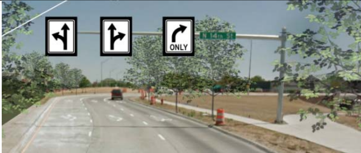
Figure 3: Overhead lane-use signing concept (oversized with black background)
