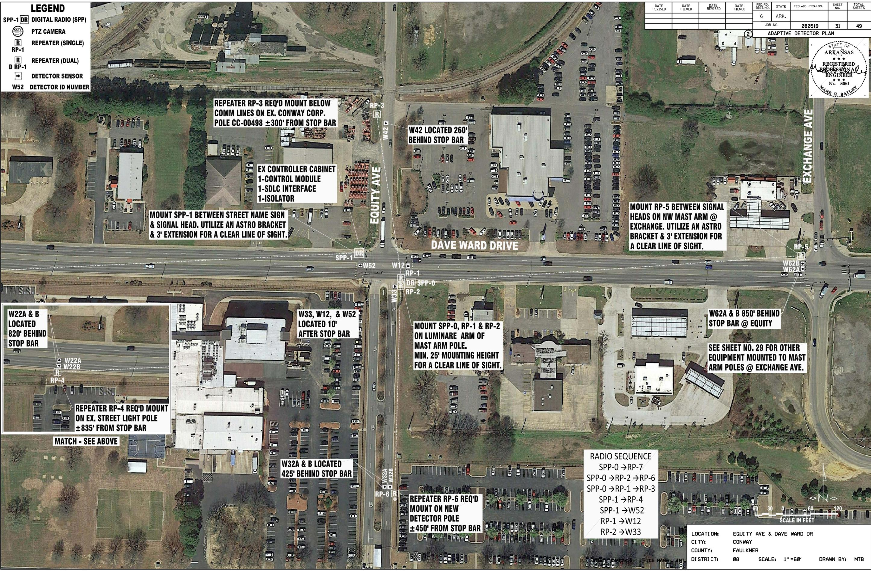
REPEATER RP-3 REQ'D MOUNT BELOW COMM LINES ON EX. CONWAY CORP. POLE CC-00498 ±300' FROM STOP BAR
