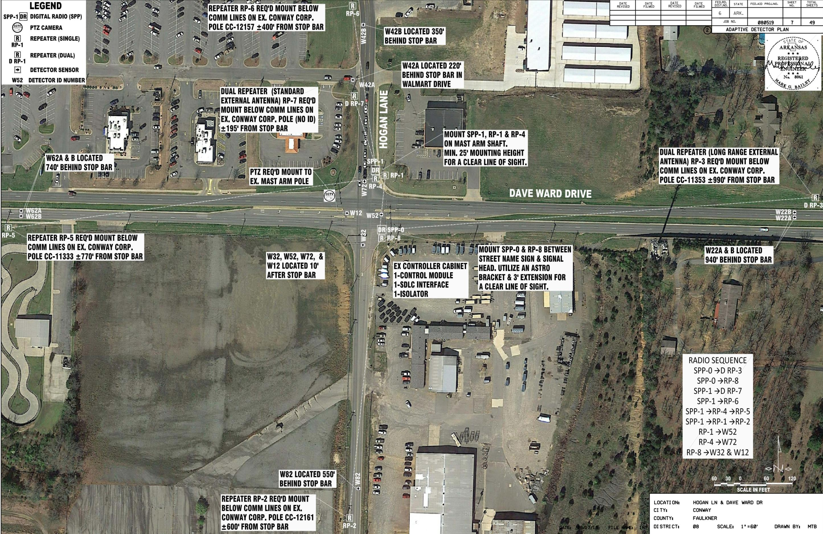
REPEATER RP-6 REQ'D MOUNT BELOW COMM LINES ON EX. CONWAY CORP. POLE CC-12157 ±400' FROM STOP BAR
