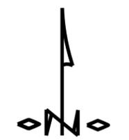
Mount SPP-1 between street name sign & signal head. Utilize an astro bracket & 3' extension for a clear line of sight.
