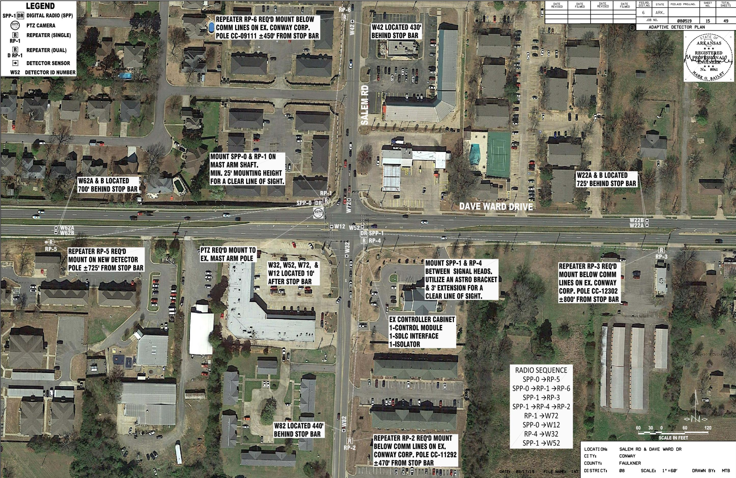
REPEATER RP-6 REQ'D MOUNT BELOW COMM LINES ON EX. CONWAY CORP. POLE CC-09111 ±450' FROM STOP BAR
