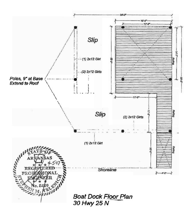
This is to certify that the planned boat dock for the Gillespie's at 30 Hwy 25 N meets 2003 LB.C. design load criteria for minimum live load of 30 psf, wind load of 20 psf, and roof live load of 16 psf.
